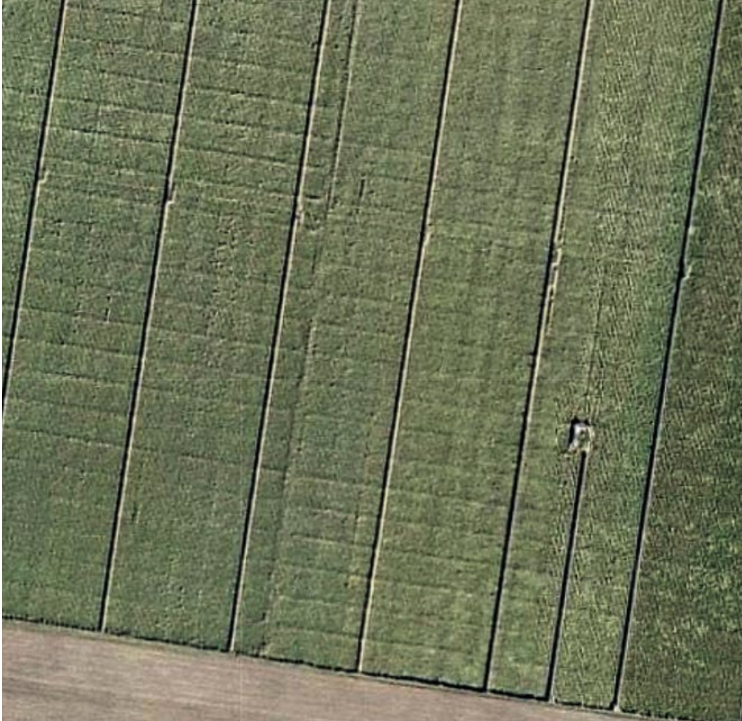
Aerial view of a cropping field after redesigning of irrigation layout (rows -top to bottom) were redesigned perpendicular to the previous configuration (left to right). The poor crop growth is clearly visible over the previous inter-row configurations (left to right).
