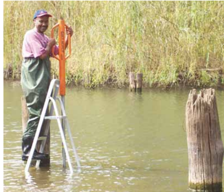
Installation of in-stream piezometers at the Kootingal transect in the Cockburn Valley.
