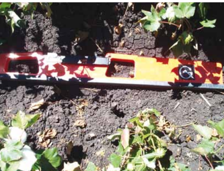
EM38 devices are an attractive tool for industry consultants and growers for precision irrigation scheduling.
