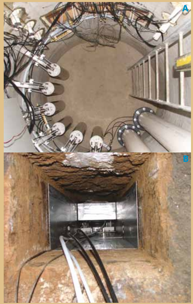
FIGURE 1: The ACRI lysimeter facility. A: View looking down into the access shaft, showing the window through which the collection trays are installed (top) and the six collection tanks into which the drainage passes for measurement (left and bottom). B: one of six collection trays during installation, showing the horizontal tunnel, drainage and vacuum tubes and space for a second tray in front. Two other pairs of trays were later installed either side of the tunnel shown.
