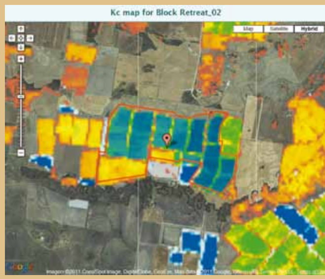
FIGURE 1: Spatial crop water use differences across irrigated cotton fields determined by IrriSAT.
