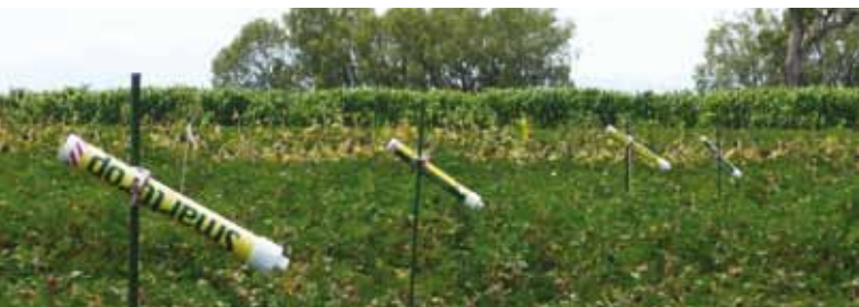
Thermal infrared sensors measuring crop canopy temperature
