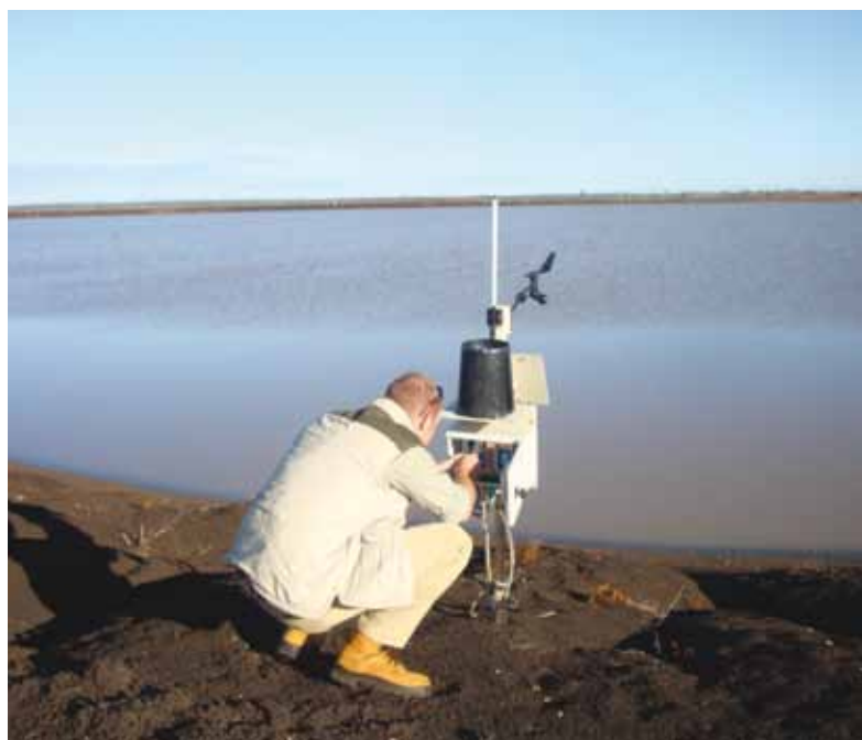
Irrimate™ Seepage and Evaporation Meter.
