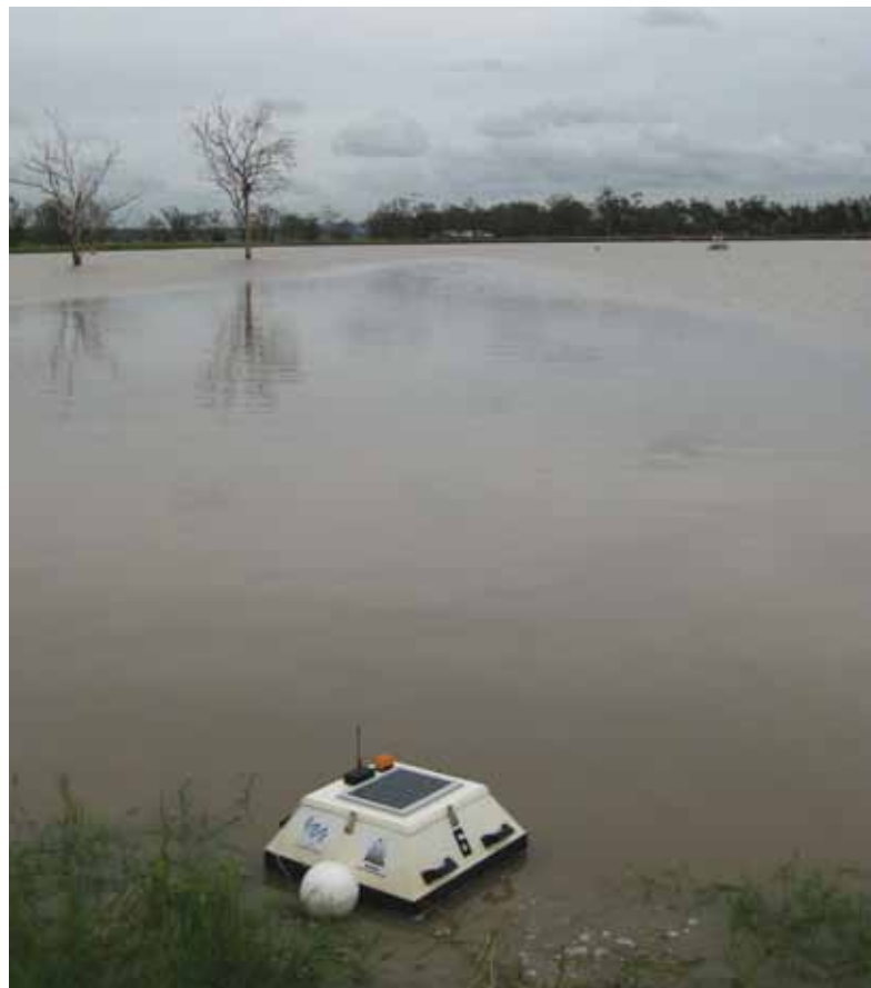
A monolayer application unit with automated dosage control works in accordance with prevailing weather conditions.
