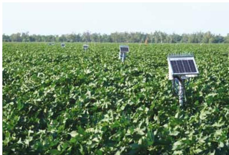
Soil moisture probes monitoring different irrigation treatments.
