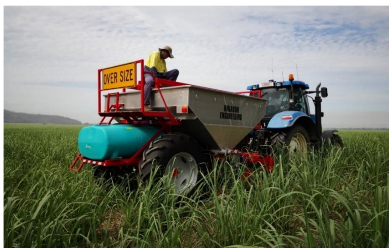
Figure 2. Application nitrogen fertilisers in the experimental plots using a variable rate fertiliser applicator at the Lilypond site.
