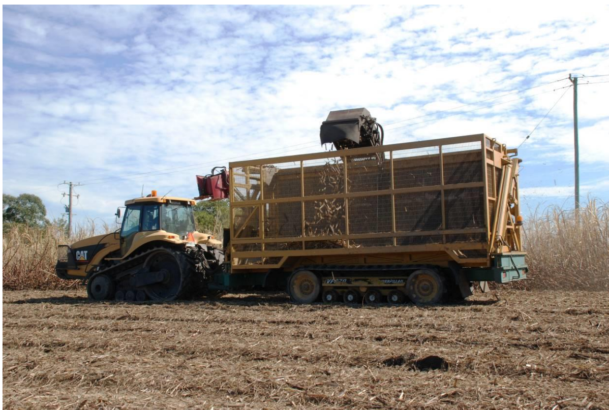
Figure 22: SRA Cat Challenger experimental plot harvester
