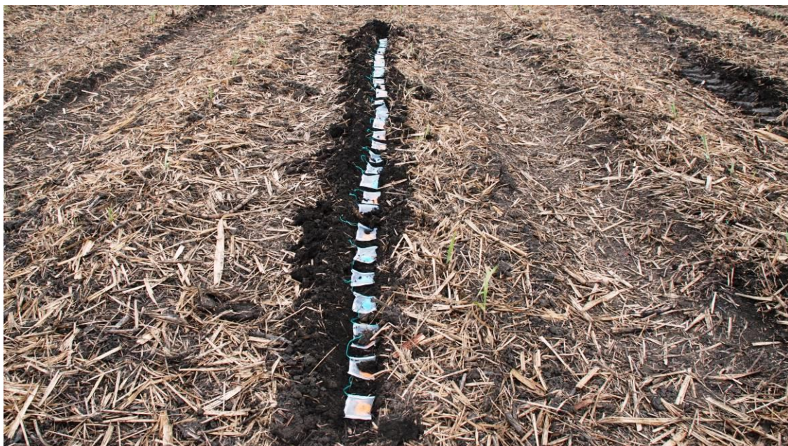
Figure 52: Mesh bag experiment in situ prior to being covered over with soil
