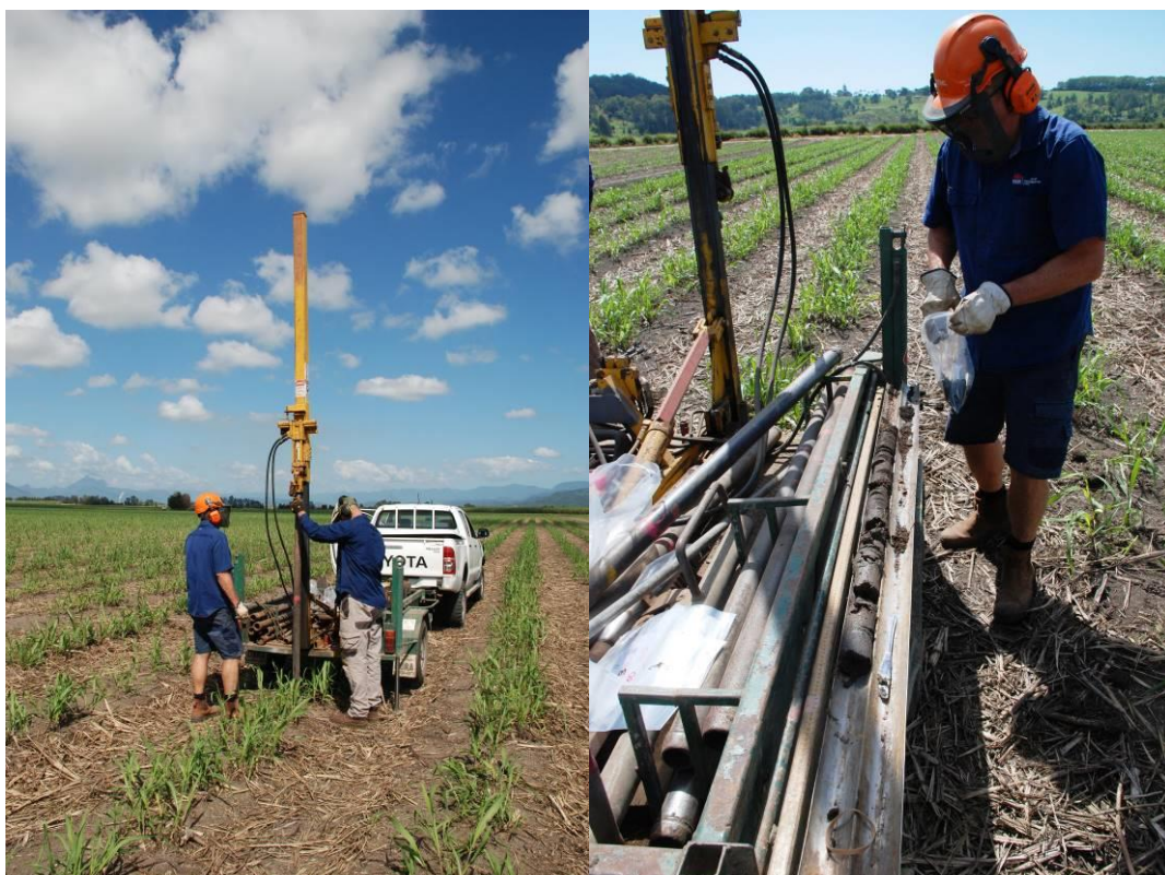
Figure 1: One metre soil core extraction using trailer-mounted hydraulic soil corer
