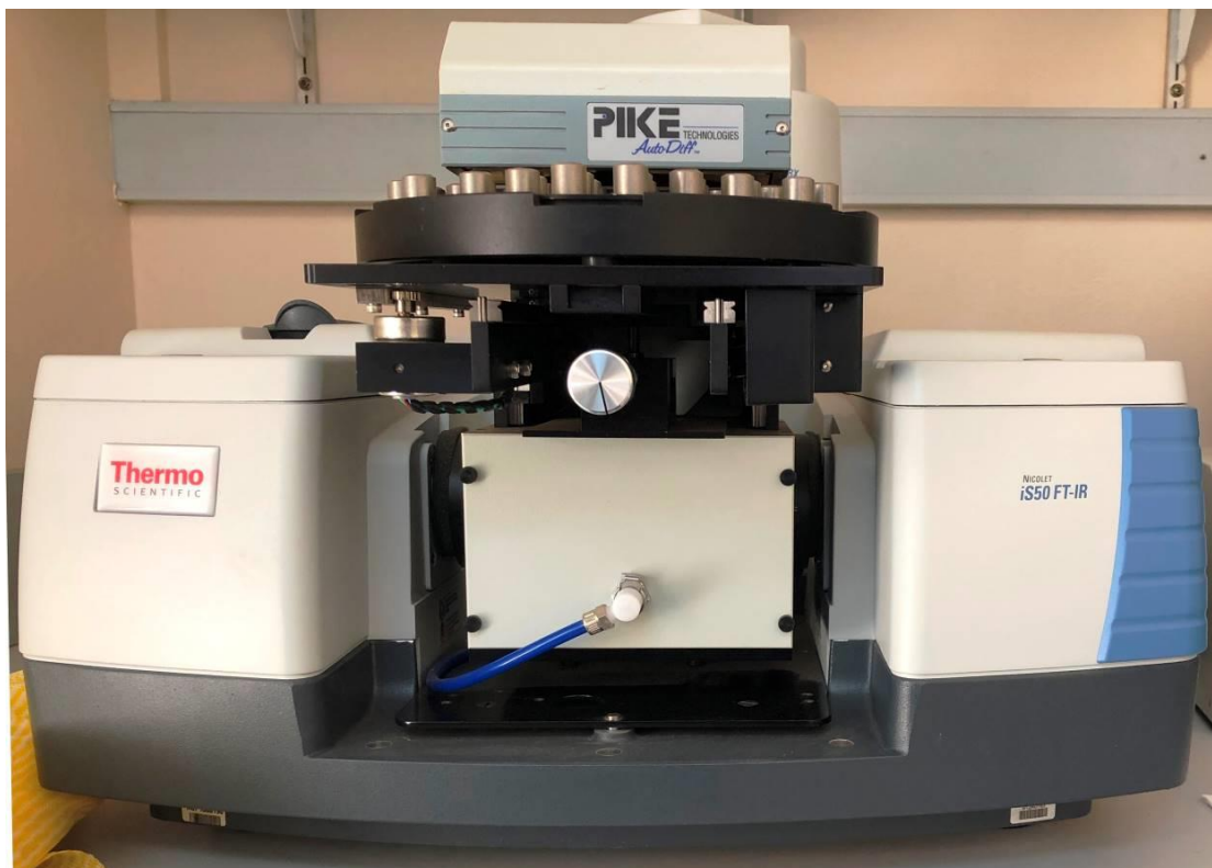
Figure 54: MIR scans were conducted on a Thermo Nicolet iS50 FTIR spectrometer
