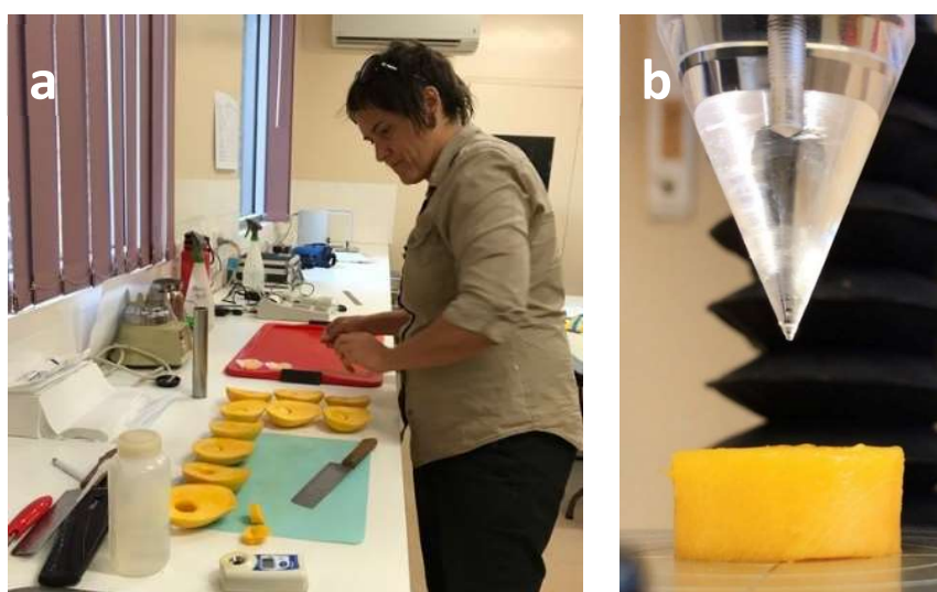
Figure C.25: To assess any post-harvest quality effects of the in-orchard nitrogen application or ripening +/- ethylene, the flesh was examined for differences in texture in 2018 and 2019. Discs of fruit being prepared for texture analysis (a). A Stable Micro Systems Texture Analyser fitted with a conical P/60C measured the force required (Newtons) for the tip of the instrument to travel 5 mm into a 10 mm deep disc of mango flesh at the rate of 2 mm s -1 (b).
