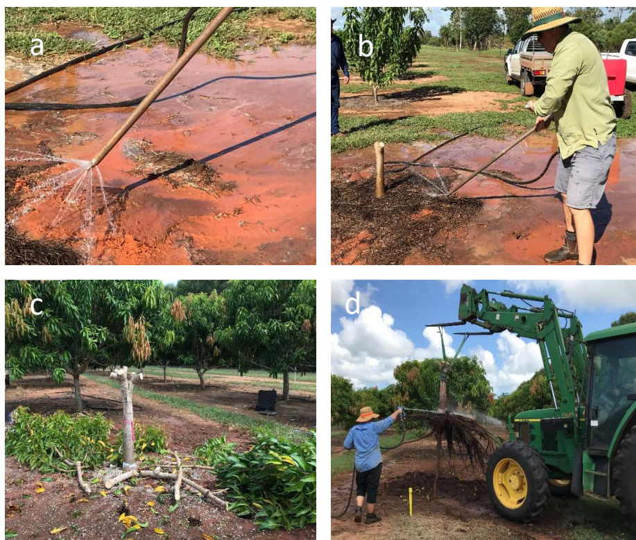
Figure C.2: A method was developed to deconstruct, then lift trees out of the soil so the component parts could be weighed and dried for analysis. A hollow steel probe with a perforated, tapered tip was attached to a fire tank with a pressure pump (a, b). Trees were de-branched with pruning saws and a chain saw (c). The probe injected large quantities of water into soil surrounding the trunk of the trees, sufficiently softening it to lift out with most roots remaining intact (d).
