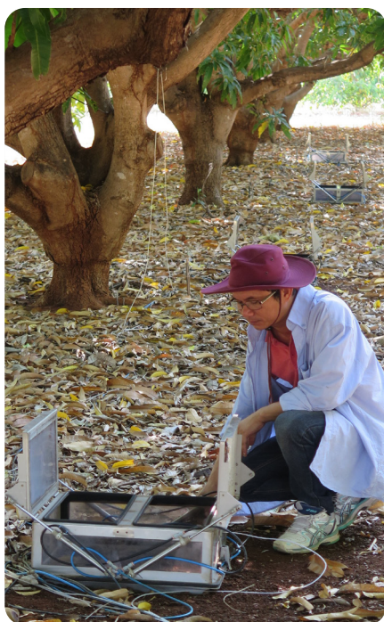
Gaseous emissions from soil, decomposing litter and fertiliser were sampled in mango orchards using automated, lidded chambers attached to a mass spectrometer. Dr Tony Asis of NT DITT checks the connections to the chambers
